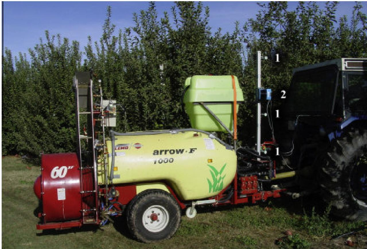
Fig. 2. Variable-rate orchard sprayer prototype implemented with three ultrasonic sensors (1) and one LIDAR sensor (2) in an apple orchard in 2005.
